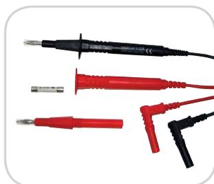
Elma 13124 safety test leads for your protection. Durable test leads with fuses in both test probes. 500mA/1000V/50kA. The test leads are double insulated, 1mm<sup>2</sup> and 1.2m long with highly insulated handles and angled banana plugs.
