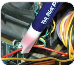
Unique forked tip for selective/accurate testing on single core cables
