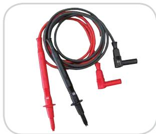
Set consisting of 1 red and 1 black extra flexible, double insulated silicone lead, 0.75 mm<sup>2</sup>, 100cm. Equipped with 4mm banana plugs with protective cover and test probe with the option of mounting alligator clips, etc.
