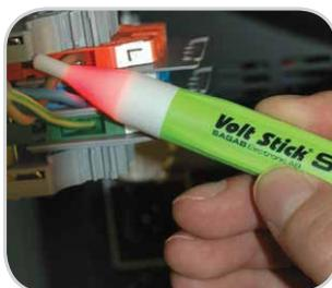
The buzzer sounds when this Volt Stick detects an AC voltage
