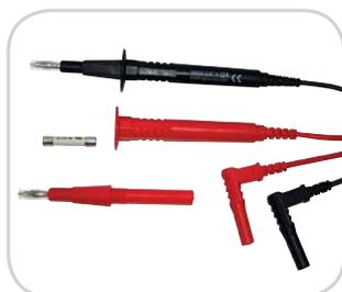
The Elma 13124 is a durable safety test lead with fuses in both test probes 500mA/1000V/50kA. The test leads are double insulated, 1mm<sup>2</sup> and 1.2m long with highly insulated handles & angled banana plugs. The test leads fulfill IEC 61010-1 CAT III 1000V and are supplied as a set of red and black.
